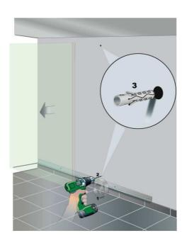
Expand the holes with the wall plug drill and insert the three plugs in the solid wall.
