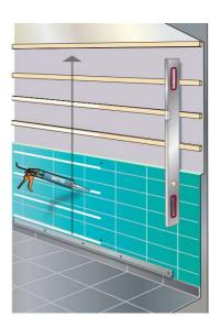
Fix horizontal studs of wood, same thickness as the tiles and apply BerryAlloc Adhesive.
