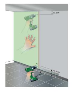
Make three small holes in the solid wall to mark the holes for the plugs (to come, illustration 3). If you use nail gun start at ill. 1 and go to ill. 4a/ 4b.
