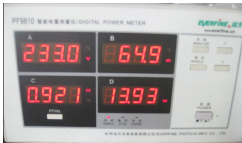
Figure5-1 Sandingled T5-SM14 Electrical Test
