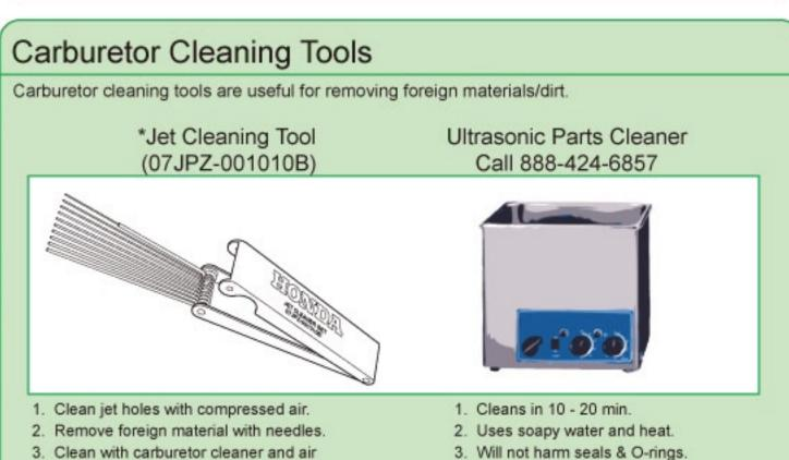
Caution: Using thick needles and applying strong force to needles will damage jets and nozzles.
