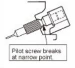
When the cap is removed, the pilot screw breaks at the narrow point, between head and thread. To remove the remaining screw, fit an appropriate rubber tube over the remaining screw and
